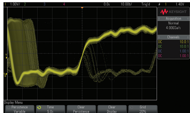
Figure 3: The Keysight MSO/DSO3000 X-Series oscilloscope reliably captures the infrequently occurring metastable state while updating at 1,000,000 waveforms per second.
